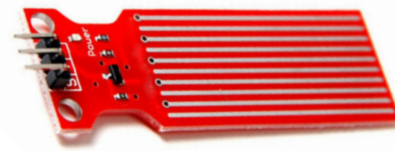
Figure 2: Water level sensor used to operate windows when it rains.
